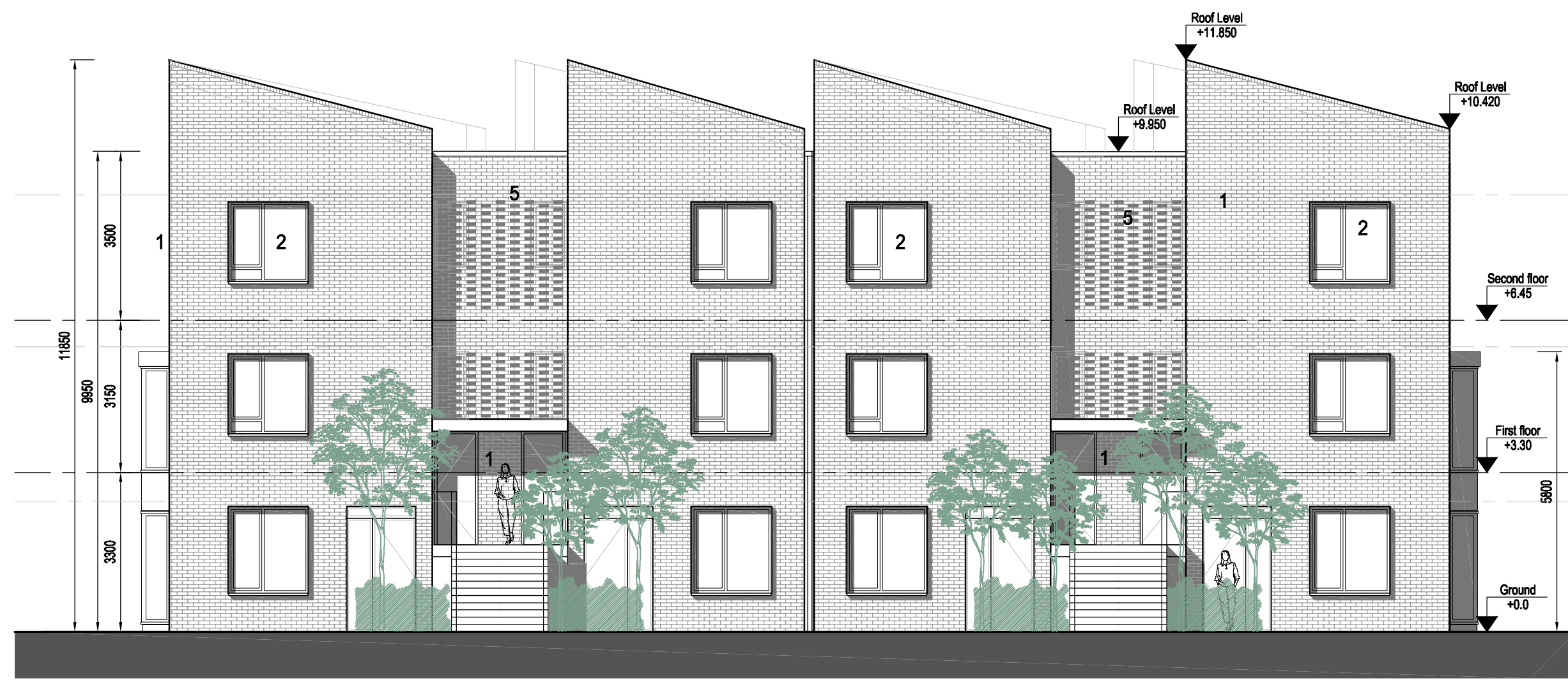
FRONT ELEVATION SCALE: 1:100 BLOCK B6 (LANDSCAPING + STORES REMOVED FOR CLARITY)
